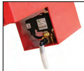
• Pressure transducer and test solenoid valve
