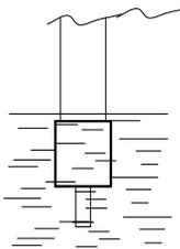
The contact is CLOSED when the float is in the liquid
