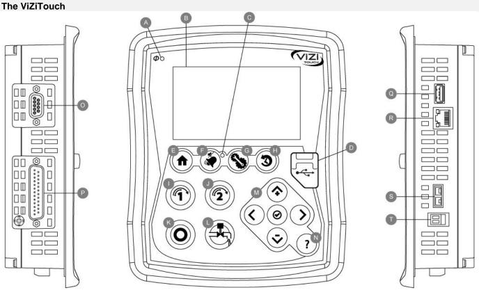
A: Power LED: Indicates if the ViZiTouch is properly powered.
