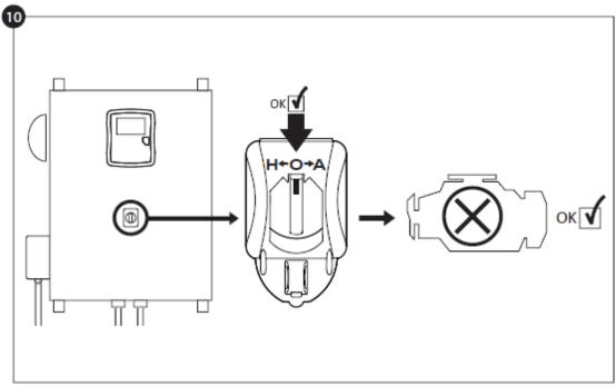
Stop the engine by turning the "Main Selector Switch" in the "OFF" position.
