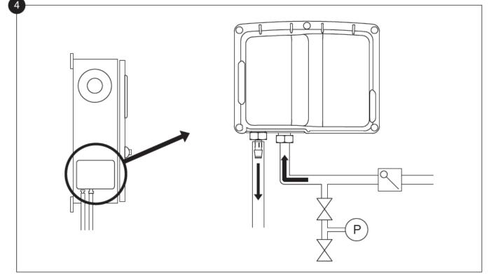
Verify and/or install the proper water connections for the water input and the drain. They must be securely installed and tightened. Refer to the silkscreen markings on the plastic cover.
