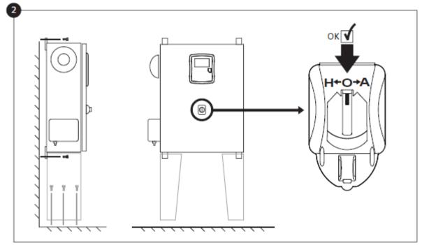
Verify that the controller is installed securely to the wall, or on the mounting stand (optional). Verify the Main Selector Switch is in the "OFF" position. This selector switch is also called the "HOA" and can be placed in 3 positions: "H" Hand/Manual, "O" OFF, "A" Automatic.
