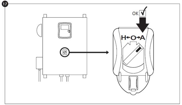
Turn the "Main Selector Switch" to the "AUTO" position. This is the preferred position and from now on, the "Main Selector Switch" should always remain in that position.
