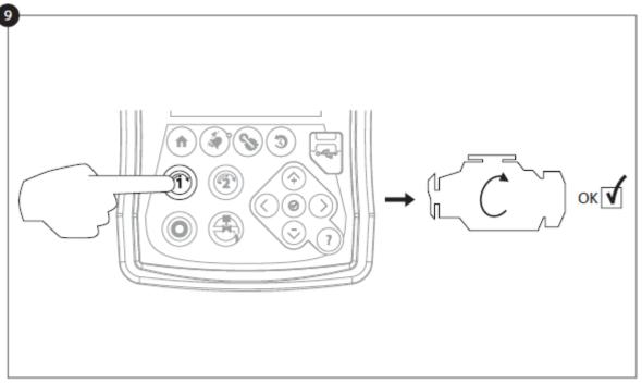
Before trying to start the engine, verify that the engine setup is complete and the exhaust pipe is connected properly. Start the engine manually by using the "Crank 1" membrane button. Verify that the engine has started and is running properly.
