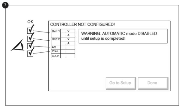
The "First Setup" page replaces the Homepage until the "First Setup" is done. Verify that the controller reads the batteries voltage and current. Verify the "AC" is "OK" and not "FAIL". Verify that the pressure reading is correct.
