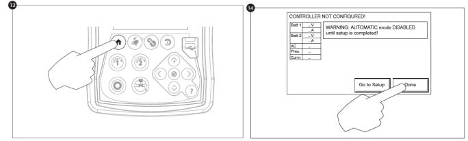
When satisfied with the controller settings, press the "Home" button on the membrane, acknowledge the changes by pressing the done button. If the done button is unavailable, ensure that a sufficient authorization code has been entered.
