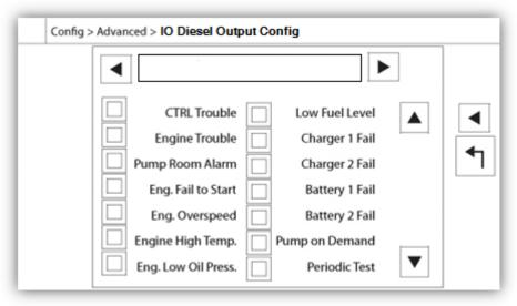
This page allows the configuration of alarm signals on the inputs, and outputs relay signals. Two buttons located far right navigates between the input and output section of the page.
