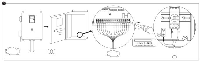
Connect all engine cables between the control panel and the controller engine terminals (Identified as "S" on the IO board diagram that is displayed in the Terminal Strip Descriptions in the manual). Secure with the appropriate torque as indicated on the torque label and verify all connections. Connect the AC main lines and ground to the AC terminals in the controller.
