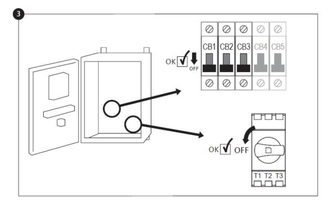
Open the controller's door and verify that the disconnect switch and all circuit breakers are in the "OFF" position.
