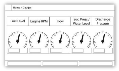
All active gauges are gathered here (ex: pressure, flow and tachometer). The discharge pressure gauge on the "Home" page must be clicked to access this page and more than 1 sensor must be installed. Clicking on the gauges will redirect to the corresponding sensor page in the advanced configuration pages. To return to the "Home" page, simply press the "Home" membrane button.
