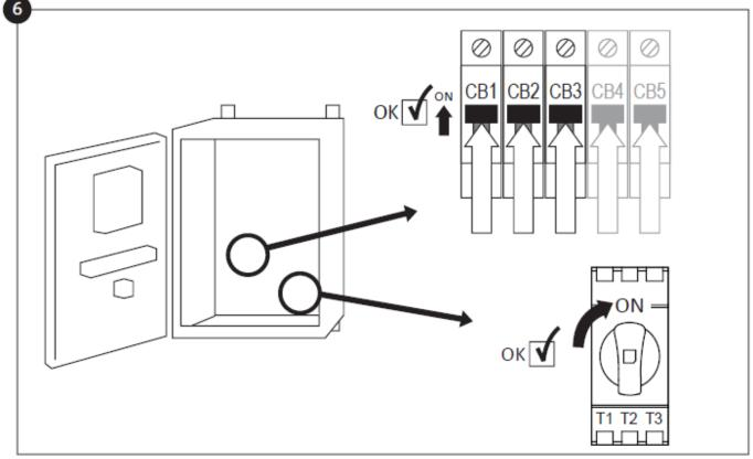
Activate the disconnect switch and all breakers by setting them to the ON position. The controller will boot up for the first time.
