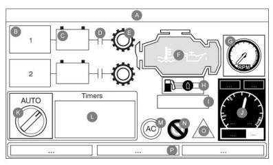
The home page displays all controller statuses and important values of the controller. All voltages, currents, pressure, engine state and status, as well as all timers and cranking sequences.
