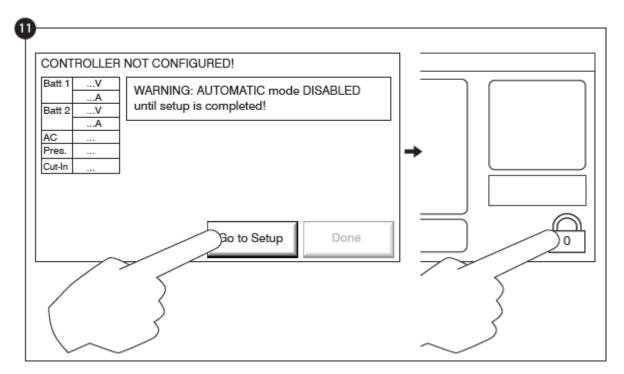
Click on the "Go to Setup" button. The "Config" page is now visible. Click on the "padlock" button to log in with your password. If needed, read the "User Login / KeyPad" section for more information on how to enter your password. Once a valid password is confirmed, the "Config" page will be visible again with the "padlock" showing that it is open the actual user security level.
