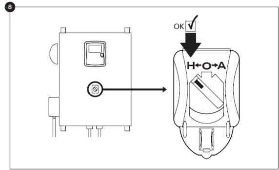
Turn the Main Selector Switch in the "HAND" position.
