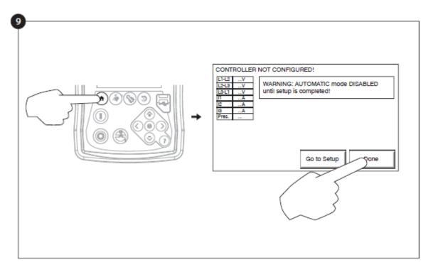
When satisfied with the controller settings, press the "Home" button on the membrane, then acknowledge the changes by pressing the "Done" button. If the "Done" button is unavailable, ensure that a sufficient authorization code has been entered and that at least all three voltages are valid.
