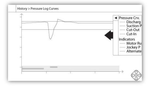
The vertical axis represents the pressure in the actual unit selected. Its scale is dynamic and will resize depending on the highest recorded value. The horizontal axis represents time and period. The left part of the horizontal axis
