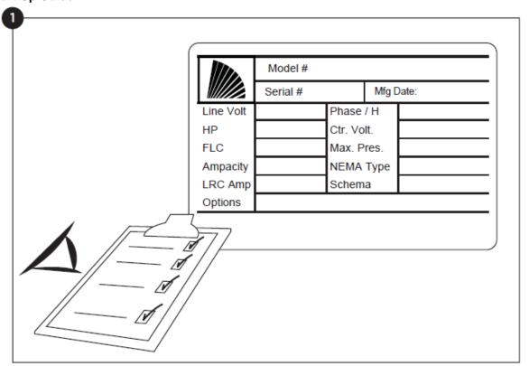
The rating label is the most important label. It must be read carefully to ensure the compatibility between the controller and the installation.
