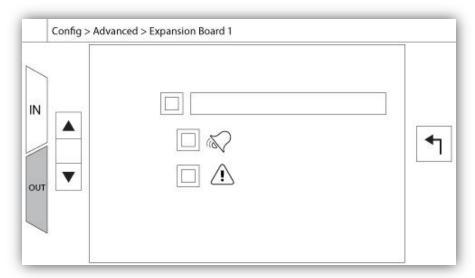
This page allows the configuration of both programmable inputs and outputs available on an IO Expansion board. Two buttons located far right navigates between the input and output section of the page.
