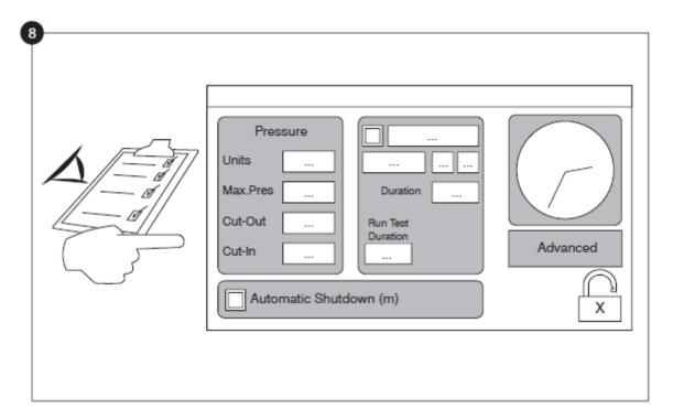
Select the controller pressure units, cut-in and cut-out. Verify that all other parameters on the setup page are correct.
