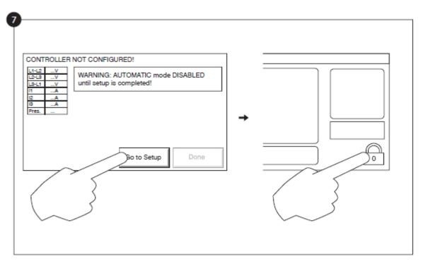
The "First Setup" page replaces the Homepage until the "First Setup" is done. Proceed to the setup page and press the lock to enter your authorization code.
