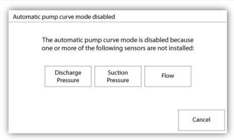
The automatic pump curve was disabled because it needs three sensors installed. The three sensors buttons link to the corresponding sensor page, allowing a quick navigation. If the button is orange, this indicates that this particular sensor is not installed. If the button is blue, it means that this particular sensor is installed. It is always possible to quit the automatic mode by pressing the "Cancel" button.
