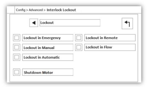
These pages allow to configure the Lockout input and the interlock output parameters. To be active, those options need to be assigned to an Input or an Output on the I/O board.
