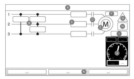
The home page displays all controller statuses and important values of the controller. All voltages, currents, pressure, motor state and status, as well as all timers and motor starting sequences.
