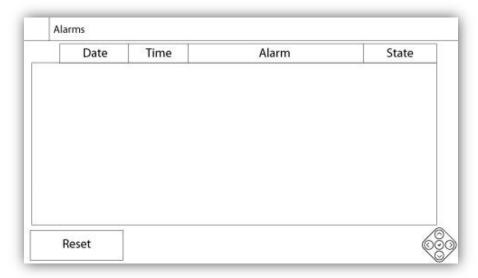
Displays the list of currently active and occurred alarms. An alarm is called ACTIVE when its triggering condition is still valid. An alarm is called OCCURRED when its triggering condition has been active, but is no longer true. Alarms representing serious concerns are colored RED. Alarms representing simple warnings are colored YELLOW. Pressing on the RESET button will reset OCCURRED alarms only. Alarms ending with \*\* are available on transfer switch models only.
