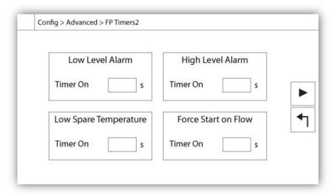
Most common timers can be configured here. Note that any timer set to 0 will remove the delay in the decision process.
