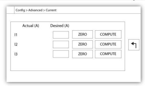
To calibrate a particular current sensing element, enter the current value as read from a calibrated ammeter and then press COMPUTE. For best results, press the ZERO button when no current is flowing through the sensing element before calibrating.
