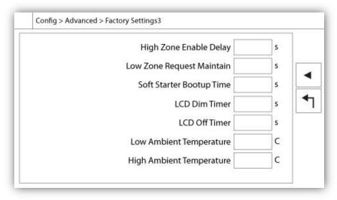
Higher Zone Enable Delay: Delay, in seconds, after which a motor run signal is sent to a higher zone controller. This option is only used for controllers in series.
