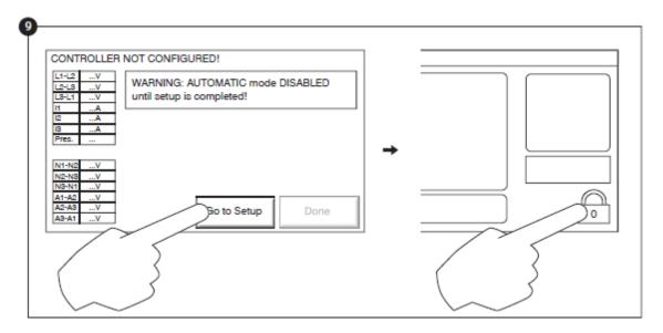
The "First Setup" page replaces the Homepage until the "First Setup" is done. Proceed to the setup page and press the lock to enter your authorization code.
