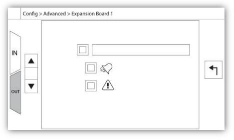
This page allows the configuration of both programmable inputs and outputs available on an IO Expansion board. Two buttons located far right navigates between the input and output section of the page.
