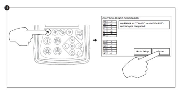
When satisfied with the controller settings, press the "Home" button on the membrane, then acknowledge the changes by pressing the "Done" button. If the "Done" button is unavailable, ensure that a sufficient authorization code has been entered and that at least all three voltages are valid.
