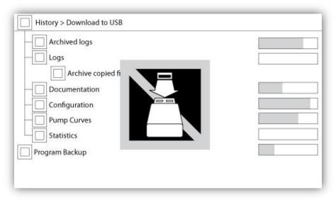
To download information from the ViZiTouch to a USB Device a user with at least a "level 1" password must be logged in. The "Download to USB" button will execute the command. If a USB Device is not present or if there is an error, a message saying "Could not mount USB drive" will appear and any further action is cancelled. To try again, remove the device, re-insert and press the button once more.
