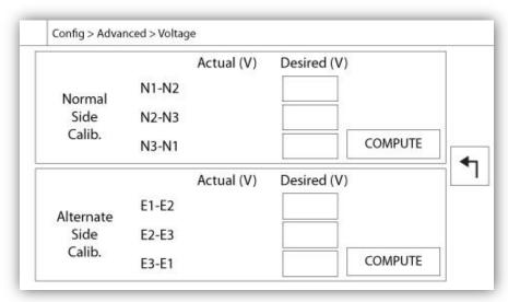
To calibrate the voltage sensing element of a power source, enter the 3 phase voltages as read on a calibrated meter then press compute. In the case of a transfer switch model, 3 additional voltages need to be calibrated the same way.
