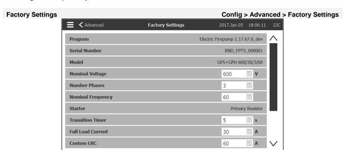
This page is used to visualize the program version, the serial number and the model of the controller.
