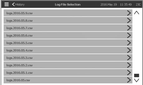
This page is used to access all past log files. Each log file is a CSV file containing the time, the date, the Cut-in, the Cut-out, the system pressure, the 3 line voltages and currents, the engine run signal, the jockey pump run signal and the log event message. Each file can contain up to 1 MB of data. The month and year are shown in the title. Each time a CSV file is full, a new one is created with an incremented number in the title. Press on the file to consult this content.
