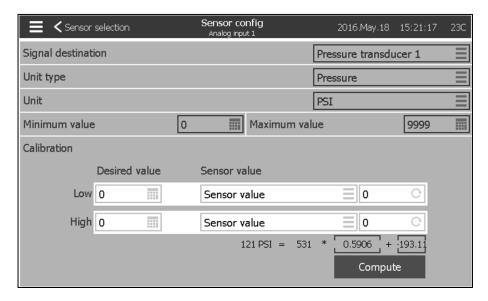
Every sensor, except the line Voltage and the Current sensor can be calibrated the same way. The Signal destination, the Unit type, the Unit, the Min and Max value are variables that are set in factory but the calibration can be made in the field.
