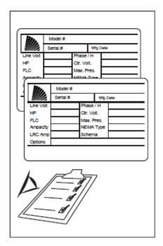
The rating label is the most important label. It must be read carefully to ensure the compatibility between the controller and the installation.
