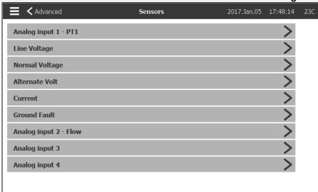
All analog sensors, voltage sensors, a current sensor and a Ground fault sensor can be calibrated by accessing this page. The Analog Input 1 is dedicated to the Pressure Transducer 1. The other Analog Input depends on the controller options.
