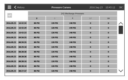
This table allows viewing of the exact values used to generate the Pressure Curves with the precise time. Pressing the blue button on the top left corner will return to the graph page.
