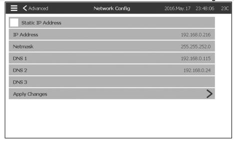
This page displays the IP address, the Subnet Mask, the Default Gateway and the DNS1-2-3 of the controller. All those parameter can be changed manually by checking the box on the upper left corner. To apply the change, press on the blue arrow in the bottom right corner.
