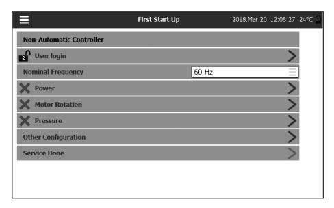
Once the controller has booted up, the "First Start Up" page appears. The controller will automatically detect and display the frequency of the power source. It is then possible to manually choose the frequency of the voltage. Press "User Login" and enter a valid authorization code. Once logged in, press "Power".
