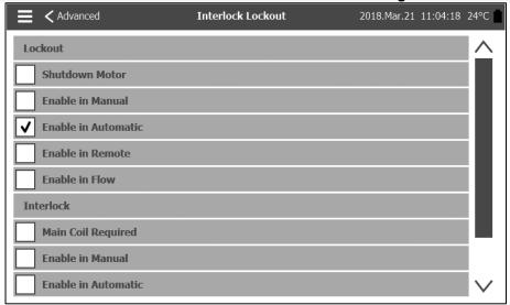
This page is used to configure the Lockout input and the Interlock output parameters. To be active those options need to be assigned to an Input or an Output on the IO board.
