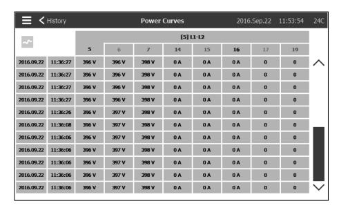
This table allows viewing of the exact values used to generate the Power Curves with the precise time. Press the blue button on the top left corner to return to the graph page.
