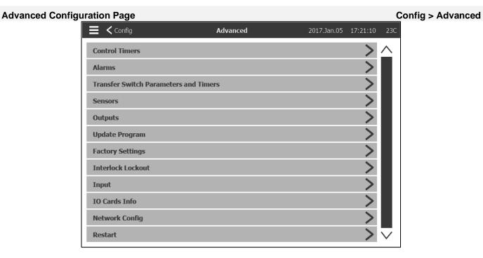
This page is the portal to all the advanced configuration parameters of the ViZiTouch. Pressing on a tab will redirect to the corresponding page.
