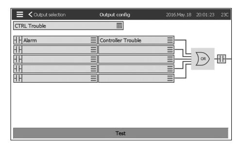
The first box from the top is used to change the name of the Output. For the output's logic, a combination of 5 digital inputs can be selected. Each input can be an alarm or a signal from a list and can be inverted by pressing the NO/NC contact symbol at the left of the screen. A logical AND or OR can combine the chosen inputs and the exit can also be inverted by pressing the NO/NC contact symbol at the right of the screen.
