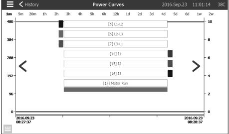
On this page, a graphic of the 3 line voltages, the 3 line currents and the motor running through time can be viewed. By pressing on the screen, the caption will disappear or will be displayed. The time scale can be changed by pressing the time span desired on top of the screen (from 1 minute to 2 weeks). The blue arrows on both sides of the graphic are used to navigate through time. The blue button in the bottom left corner leads to the table used to generate this graph.
