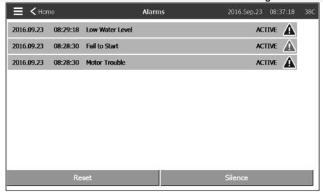
Displays the list of currently active and occurred alarms. An alarm is called ACTIVE when its triggering condition is still valid. An alarm is called OCCURRED when its triggering condition has been active, but is no longer true. Alarms representing serious concerns are colored RED. Alarms representing simple warnings are colored YELLOW. Pressing on the RESET button will reset OCCURRED alarms only. Alarms ending with \*\* are available on transfer switch models only.
