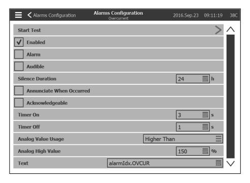
Start Test: The alarm can be tested using this button. This test will only announce the chosen alarm. It will activate the bell if the alarm is audible and will activate any output relays associated with this alarm. The test will not activate other common alarms or other components. To stop the testing, press the "Stop Test" button.
