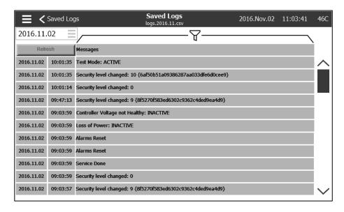
The logs are arranged chronologically. To select the displayed data, press on the filter icon in the top center of the screen.
