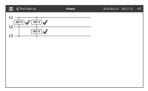
Verify that the normal voltage shown at L1-L2, L2-L3 and L1-L3 (nominal) is the same as what is written on the fire pump controllers nameplate. The fire pump controller will validate the nominal voltage automatically versus what it has been built for.
