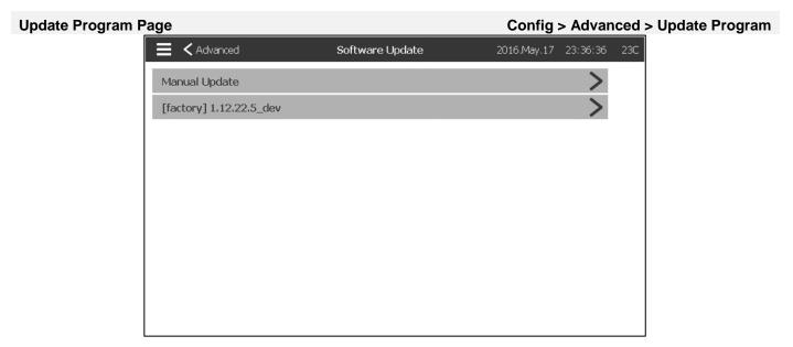
This page is used to update the controller software. A USB key or a network connection with the software update is needed.
