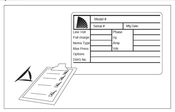
The rating label is the most important label. It must be read carefully to ensure the compatibility between the controller and the installation.
