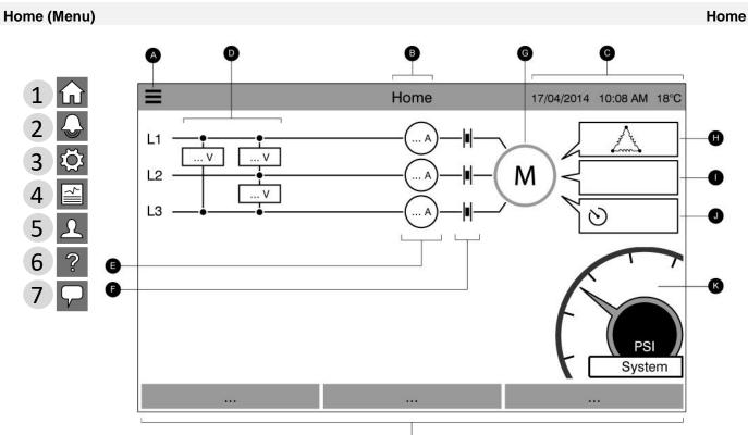
The home page displays all controller statuses and important values of the controller. This includes all voltages, currents, pressures, motor state and status, as well as all timers and motor starting sequences.
