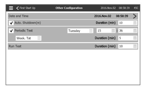
Go back to the controller start-up page and press the "Other Configuration" button. Enter the time and date. Select the "Automatic shutdown" and the duration the pump will keep running after the automatic stop is desired. Select the frequency at which the periodic test will occur, the day of the week, the hour and the duration of the test. Also, enter the duration of the Manual Run Test.
