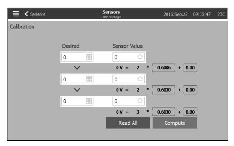
To calibrate the line voltage sensor, use an external voltmeter that is already calibrated. With the control panel under power:
