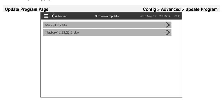
This page is used to update the controller software. A USB key or a network connection with the software update is needed.
