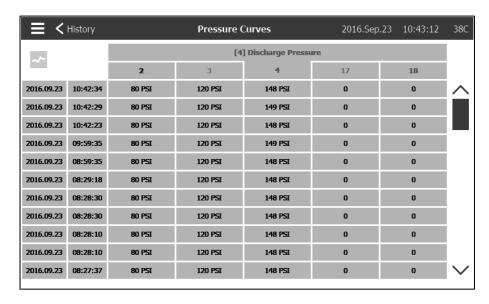
This table allows viewing of the exact values used to generate the Pressure Curves with the precise time. Pressing the blue button on the top left corner will return to the graph page.
