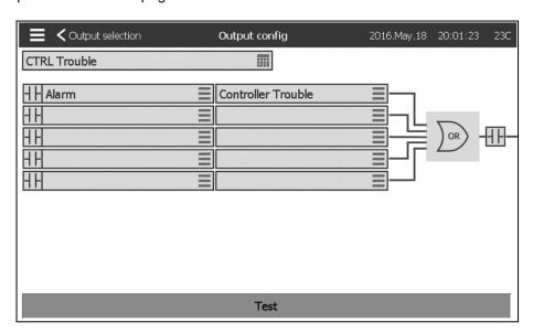
The first box from the top is used to change the name of the Output. For the output's logic, a combination of 5 digital inputs can be selected. Each input can be an alarm or a signal from a list and can be inverted by pressing the
