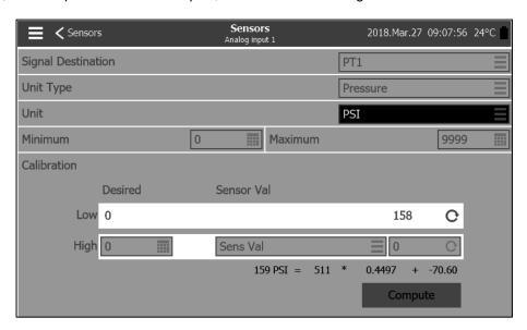
For the pressure transducer PT1, the low point (zero) is automatically acquired during first power up. It can be reacquired by pressing the blue round arrow. The high point needs to be entered in order to calibrate the sensor.
