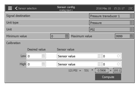
Every sensor, except the line Voltage and the Current sensor can be calibrated the same way. The Signal destination, the Unit type, the Unit, the Min and Max value are variables that are set in factory but the calibration can be made in the field.
