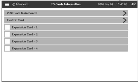
This page is used to visualize the ViZitouch and the IO Card registers by pressing on the blue arrows on the right of the screen. Expansion Cards can also be installed via this page.
