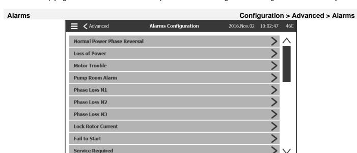
Most alarms are not configurable in the field, but some are with the appropriate password level. If it's configurable, the checkboxes will be in white. Otherwise the checkboxes will be grey. Also, the two last fields: Value Usage and Analog Value are not always visible.
