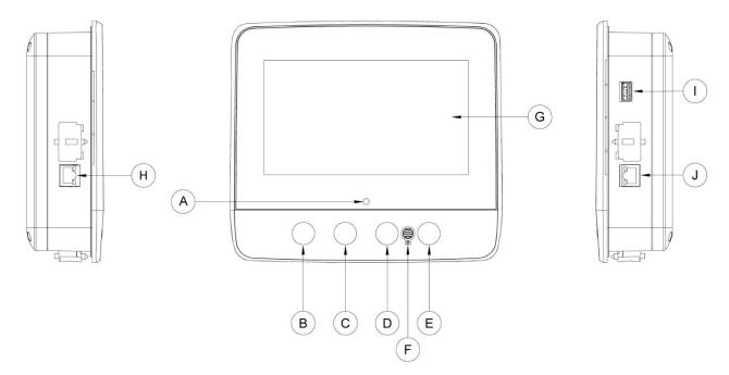
A: Power LED 3 colors: Pulsing green if the ViZiTouch is properly powered.
