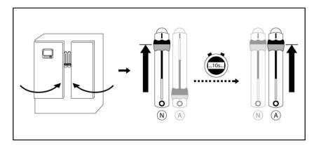
Secure the doors in the closed position then put the normal power circuit breaker disconnecting means in the ON position. Wait 10 seconds for the controller to load correctly, then put the alternate power circuit breaker disconnecting means to the ON position. Verify the readings on the controller main screen.
