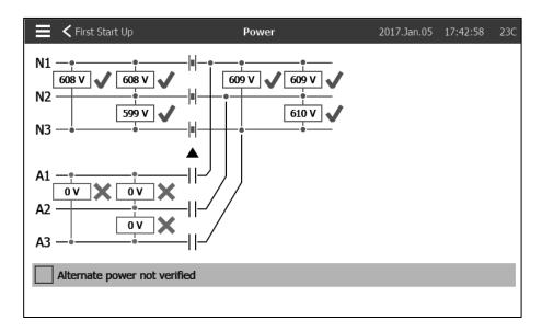
This page is used to verify the supply voltage. It displays the voltage that the controller reads between each phases for the "Line Voltage", the "Normal Voltage" (N1-N2-N3) and the "Alternate Voltage" (A1-A2-A3).
