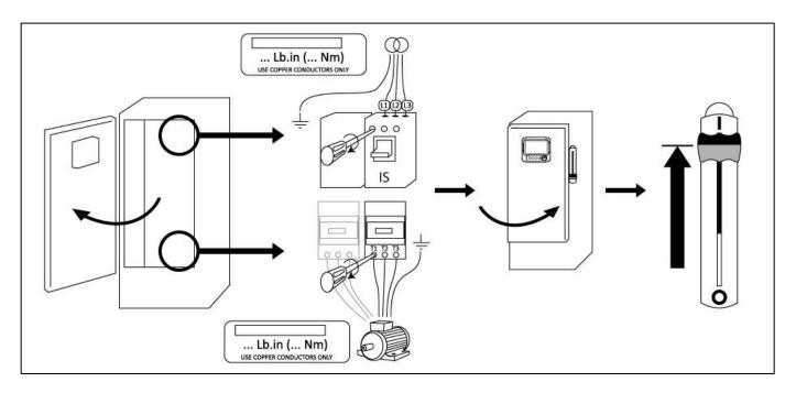
Connect the input power and the motor on their respective terminals. Secure with the appropriate torque as indicated on the torque label and verify all connections. Secure the door in closed position then put the circuit breaker disconnecting means in ON position. Verify the readings on the controller main screen.
