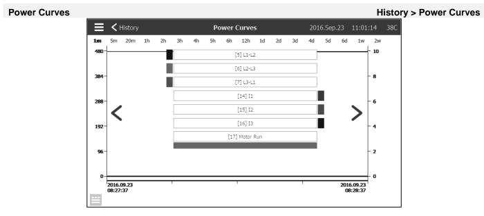
On this page, a graphic of the 3 line voltages, the 3 line currents and the motor running through time can be viewed. By pressing on the screen, the caption will disappear or will be displayed. The time scale can be changed by pressing the time span desired on top of the screen (from 1 minute to 2 weeks). The blue arrows on both sides of the graphic are used to navigate through time. The blue button in the bottom left corner leads to the table used to generate this graph.
