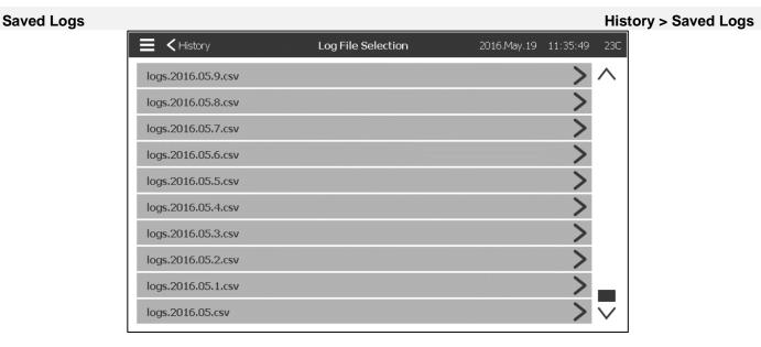
This page is used to access all past log files. Each log file is a CSV file containing the time, the date, the Cut-in, the Cut-out, the system pressure, the 3 line voltages and currents, the engine run signal, the jockey pump run signal and the log event message. Each file can contain up to 1 MB of data. The month and year are shown in the title. Each time a CSV file is full, a new one is created with an incremented number in the title. Press on the file to consult this content.
