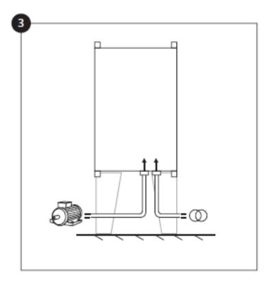
Make sure to drill holes for the motor and power connections and run the cables inside the panel, all in accordance with the specifications in order to minimize interference with other equipment.
