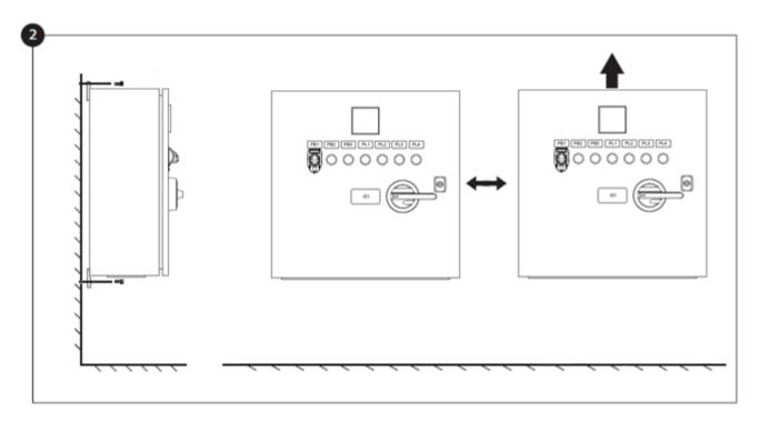
Verify that the controller is installed securely on the wall.
