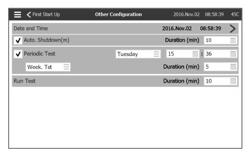
Go back to the controller start-up page and press the "Other Configuration" button. Enter the time and date. Select the "Automatic shutdown" and the duration the pump will keep running after the automatic stop is desired. Select the frequency at which the periodic test will occur, the day of the week, the hour and the duration of the test. Also, enter the duration of the Manual Run Test.
