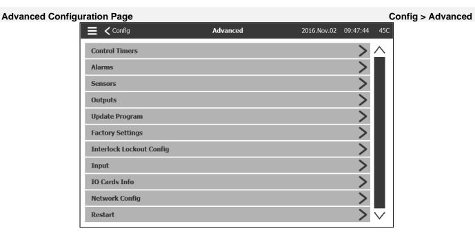
This page is the portal to all the advanced configuration parameters of the ViZiTouch. Pressing on a tab will redirect to the corresponding page.
