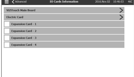
This page is used to visualize the ViZitouch and the IO Card registers by pressing on the blue arrows on the right of the screen. Expansion Cards can also be installed via this page.
