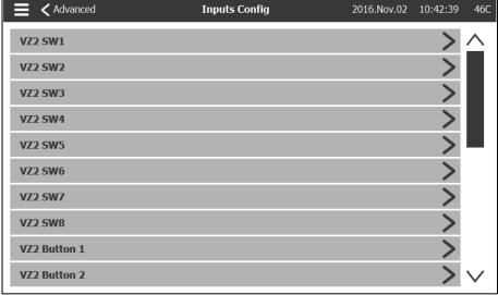
This page is for vizualisation purpose only. It allow the user to verify which signal is mapped on which controller's input.
