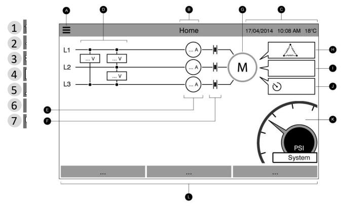
The home page displays all controller statuses and important values of the controller. This includes all voltages, currents, pressures, motor state and status, as well as all timers and motor starting sequences.
