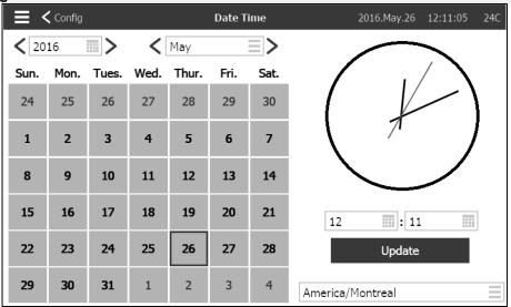
Select the Year by pressing inside the year box and enter the value, or use the left and right arrows to simply decrement or increment the value. Likewise, select the month by pressing on the month box and select the value from the list shown, or use the left and right arrows to cycle through the choices.
