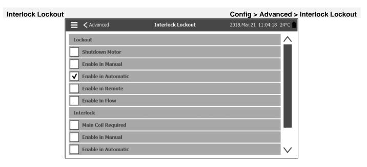
This page is used to configure the Lockout input and the Interlock output parameters. To be active those options need to be assigned to an Input or an Output on the IO board.
