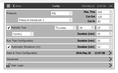
The main configuration page is used to setup all basic configuration parameters and provides a quick means of changing the most common settings.
