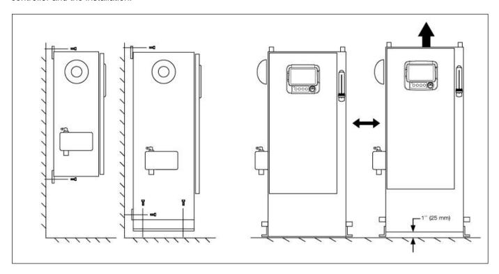
Verify that the controller is installed securely on the wall, or optionally on the mounting stand.
