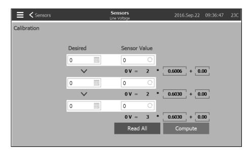
To calibrate the line voltage sensor, use an external voltmeter that is already calibrated. With the control panel under power:
