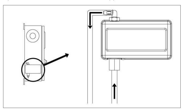
Verify and/or install the proper water connections for the water input and the drain. They must be securely installed and tightened. Refer to the silkscreen markings on the plastic cover.
