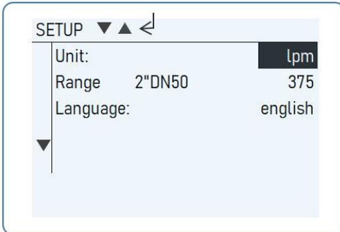
After that, changes can be made within the range of values available using the “ON” or middle key.
