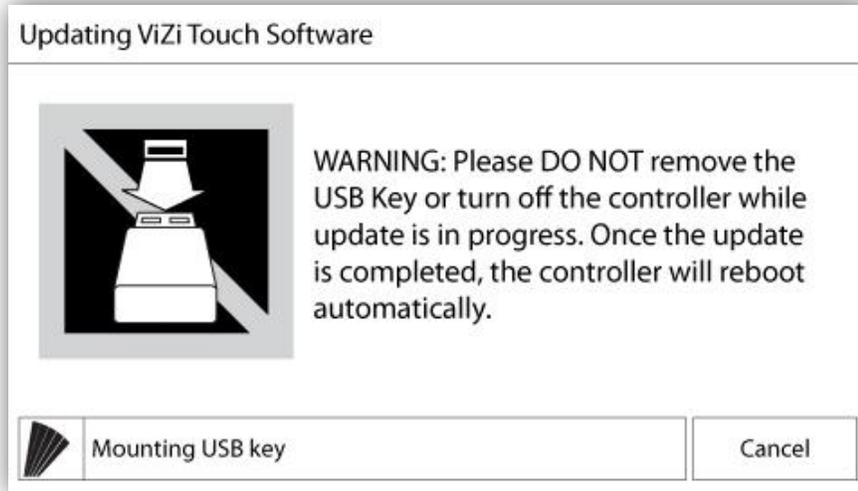
This procedure is highly important and must be attempted with care. Please make sure to contact the factory prior to using the Update Software function.
