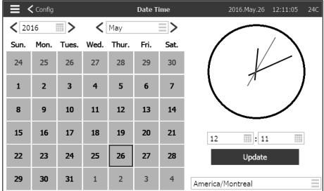
Select the Year by pressing inside the year box and enter the value, or use the left and right arrows to simply decrement or increment the value. Likewise, select the month by pressing on the month box and select the value from the list shown, or use the left and right arrows to cycle through the choices.
