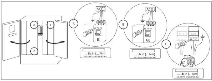
Connect the normal input power, the alternate input power and the motor on their respective terminals. Secure with the appropriate torque as indicated on the torque label and verify all connections.
