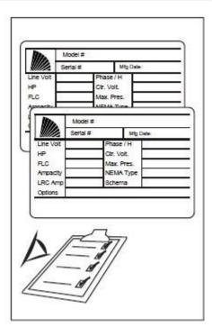
The rating label is the most important label. It must be read carefully to ensure the compatibility between the controller and the installation.
