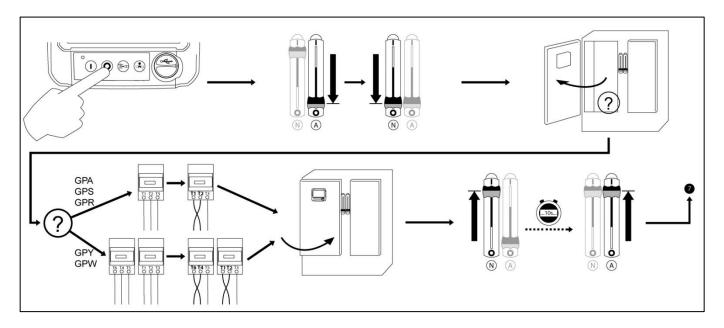
Once the motor rotation has been checked, go back to the controller start-up page and press the "Verify pressure" button.
