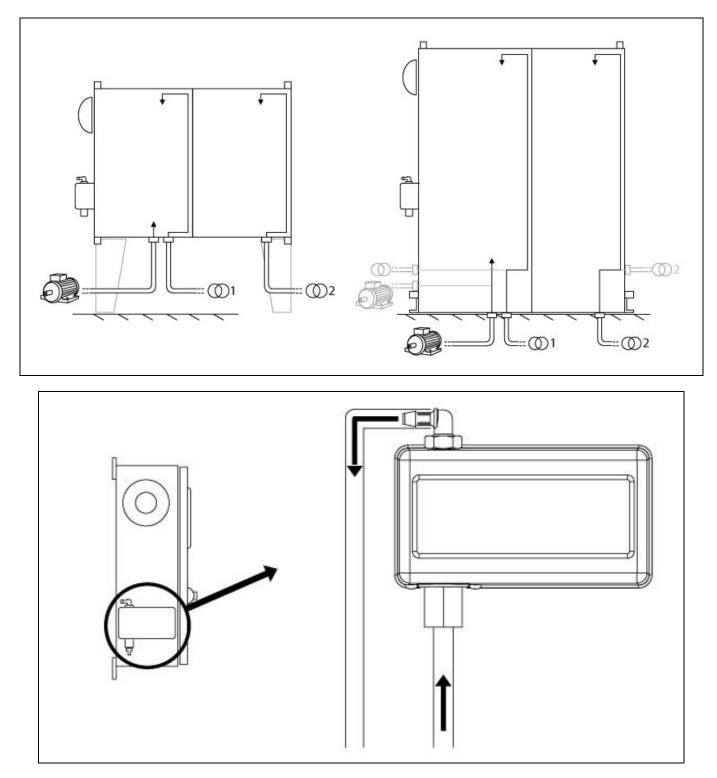
Verify and/or install the proper water connections for the water input and the drain. They must be securely installed and tightened. Refer to the silkscreen markings on the plastic cover.
