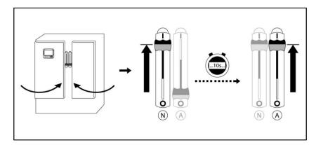
Secure the doors in the closed position then put the normal power circuit breaker disconnecting means in the ON position. Wait 10 seconds for the controller to load correctly, then put the alternate power circuit breaker disconnecting means to the ON position. Verify the readings on the controller main screen.
