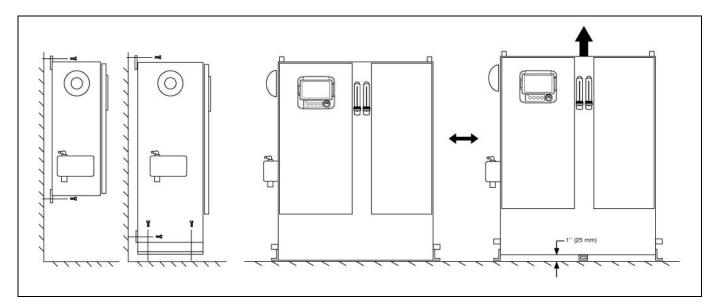
Verify that the controller is installed securely on the wall, or optionally on the mounting stand.
