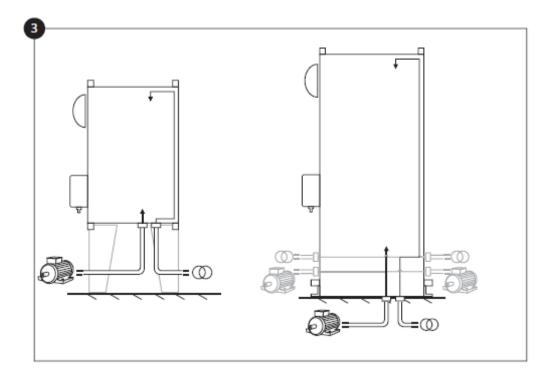
Make sure to drill holes for the motor and power connections and run the cables inside the panel, all in accordance with the specifications in order to minimize interference with other equipment.
