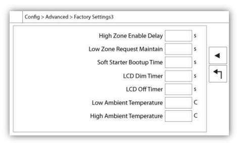
The factory settings are always pre-configured at the factory and set the main parameters of the controller. Most of the settings found on this page can only be changed by an authorized Tornatech employee and is protected by a
