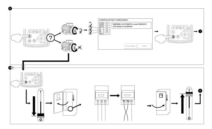
Verify the motor rotation to ensure that the pump is turning in the right direction. The START and STOP push buttons can be used to toggle the motor ON/OFF.
