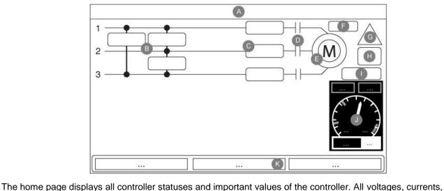
Alarm indicator: Exclamation mark in a red triangle icon. As soon as at least one alarm is ACTIVE or OCCURRED, the alarm indicator will be flashing.
