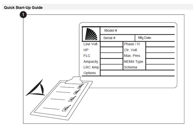
The rating label is the most important label. It must be read carefully to ensure the compatibility between the controller and the installation.
